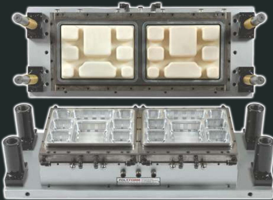
Trim-in-place thermoforming mould with 2 cavities (2 trays at-a-time) for 8-compartment Meal Tray
