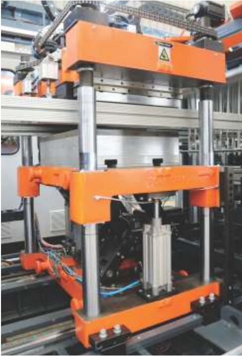
Forming and cutting station in solid steel cast structure with needle bearings for toggles
